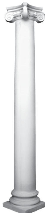
APC5 (Col) 3.210 m HIGH 254 mm DIAMETER 360 x 360 mm BASE
